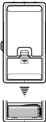
When the battery runs low, the display indicates "LOW BATT". Install a new battery as soon as possible. When the battery is completely depleted, the display goes dark and the sound is no longer output.
